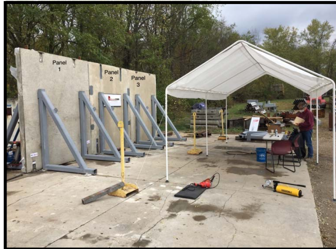
(b) Panels after installation of lateral braces
